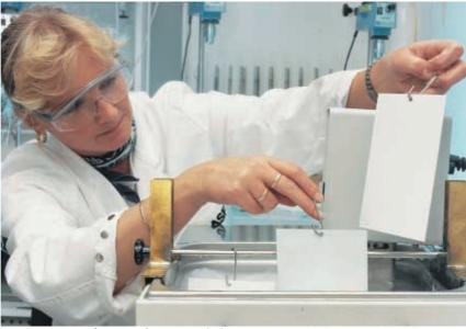
Performance of a caustic soda detergent test at BASF Coatings AG.
